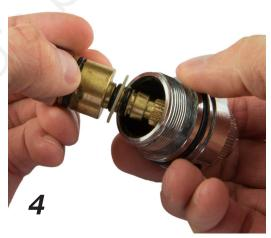
Once clip is removed, you can push or tap out shaft as shown.
