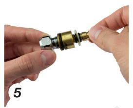
Unthread the shaft into two parts.
