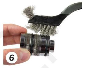
Use a brush and a solvent to thoroughly clean the cartridge. Do not use too strong of a solvent as it could melt the rubber gaskets.
