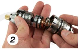
When done unthreading, the top and bottom can be separated. Disassemble as shown, taking care not to drop, lose, or damage any parts.
