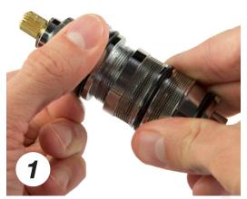
Using a pair of channel locks, grasp the cartridge at the top and bottom. Do not grasp by the rubber gaskets as this will damage them and cause leaks. Loosen by turning the locks against each other. Once loosened, the top and bottom can be unthreaded by hand.
