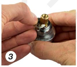
Gently remove the locking clip at the top. If unable to remove by hand, use a small flat-head screwdriver or needle-nosed pliers.
