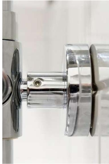
The shower column is attached to the wall with either a short or long pipe connector. The long pipe can range between 9 3/4" to 10 3/4". The short pipe can range between 2 1/4" to 3 1/4". These two images show a short pipe connector.
