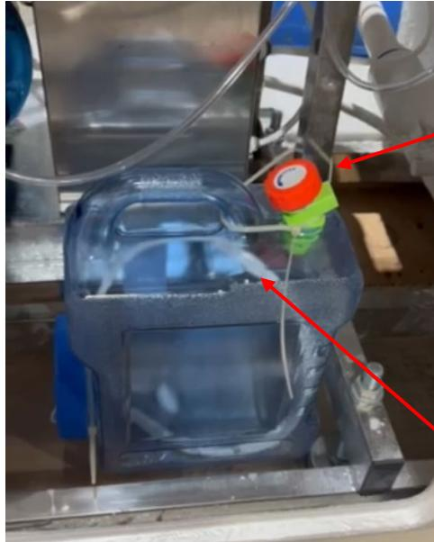
Cut the Ties and remove the container from under the tub
