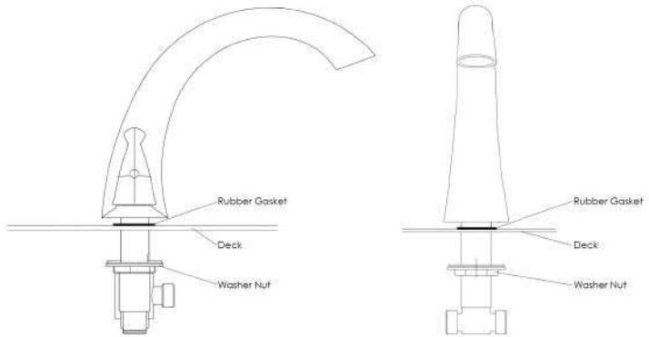
**2.** Unscrew the washer nut and place the rubber gasket and spout above the deck. After, secure the washer nut from underneath the deck.
