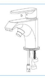
Step.2 Use an Allen wrench to remove the handle Screw.
