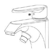
Step.3 Take out the handle and remove the brass escutcheon
